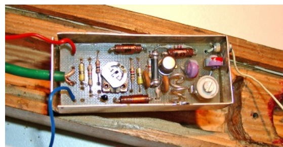
A 31211-6 bug, microphone and battery compartment hidden in a hollow wooden lath. (Above). This assembly could be fitted under a table or wooden furniture.
